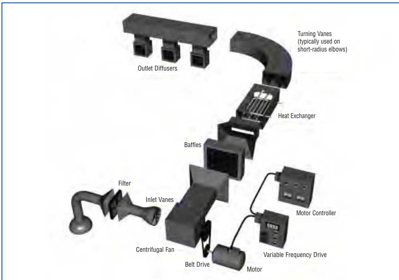
Figure 1-3. Example Fan System Components
